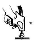
Clip Pins are permanently welded in position flush with insulation.
