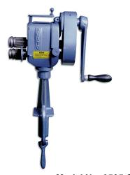
The 0585 is furnished with Ogee Bead Rolls and Crimping Rolls for combined crimping and beading operation. By replacing Beading Rolls with Spacing Collars (regularly furnished) the machine can be used for crimping only. 3/8" or 1/2" Single Bead Rolls are available for beading only. This machine is adjustable for deep or shallow bead and for "fade-away" crimp. The 0585 comes complete with #975 Bench Standard and Spanner Wrench.
